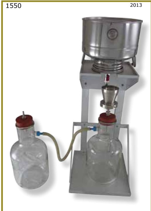
Metallic structure conforming to method, metallic filter funnel supported by a base with support for closing of the tightness membrane, 5 litres filling container made in stainless steel with stopper for spillage, one receiving and one security 5 litres filtering flask. Connection flaske to flaske by vacuum tube nad the flask are provided with grounding system. Rubber stoppers and tubes for connection.
